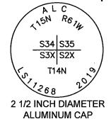
**NE S34** 2 1/2" ALUM. CAP "LS11268" -GATE 5.34 THIS CORNER 5.34 SET 2 1/2" ALUM. CAP "LS11268" | *S.35 S.33* T. 15N. N89**'**49'52 5304.89 T. 14N. SW S34 2 1/2" ALUM, CAP "I S11268"
